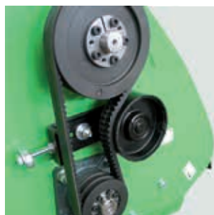
Facile tensione cinghie. Easy belts tightening adjustment.
